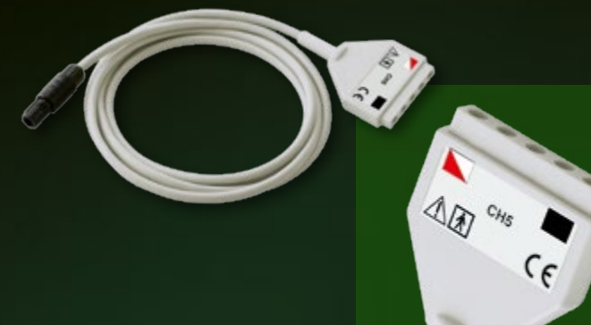
41-0083 Stimulation cable for TWISTER® MM 1-channel, output 5-6, for connection of stimulation probes and electrodes, with DIN 42802-1 connectors, cable length 4 m, connector black/black, not autoclavable
