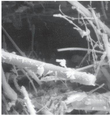
macrophotograph of the filter surface showing deposited contaminants
