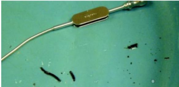
The problem: Debris found inside a reusable suction tube after cleaning and sterilization
