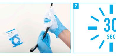
Step 7 - Place the probe in the 'clean' area and leave it for 30 seconds.
