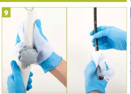
Step 9 - Rinse the probe to remove excess disinfectant.
