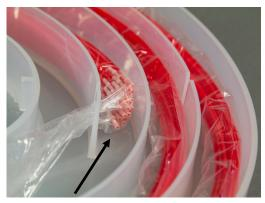
3. Insert the sealed end of the refill pack into one of the V slots. Pick the one suitable for the brush length..
