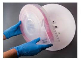
4. Place the loaded cassette onto the mounting plate.
